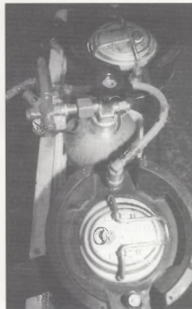
(Above) Each unit is comprised of one 5-pound CO2 container and four 5-gallon stainless steel canisters, and a pre-set pressure regulator (40 psi). Each unit contains a double canister pressure hose assembly, spray hose and handgun.
