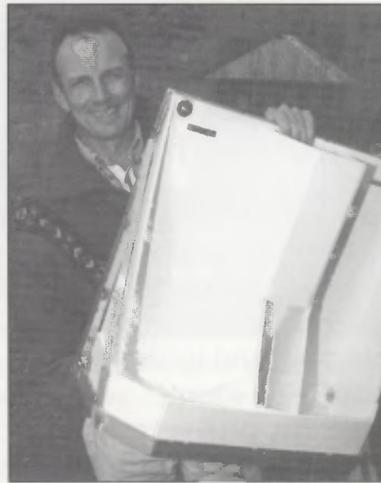
After several prototypes, this aluminum frame pannier lined with lightweight, corrugated, and waterproof plastic proved best.
