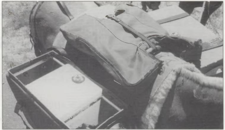
Tom Henderson (left) uses a system that mounts two 5-gallon electric battery-operated sprayers mounted in Ralide Horsepac panniers (above). These units are totally self-contained and feature stainless steel ball lock disconnects pre-set pressure regulators. The herbicide tanks feature bottom drain valves and spray is pumped from each unit equally so loads stay balanced on the pack animal throughout the day.
