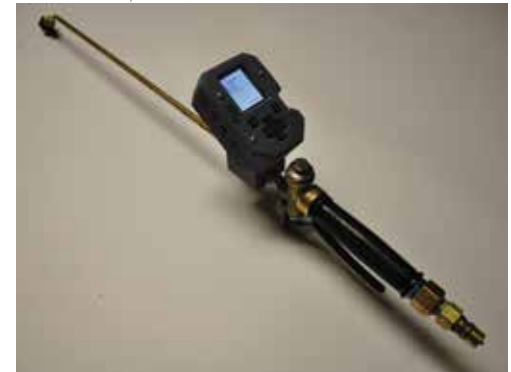
THE “SMART” SPRAY WAND records GPS location, herbicide flow, application time and other desired data. It can simplify invasive weed management and has provided the necessary data capture for the development of a weed treatment cost model.
